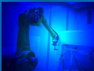
**Part Trimming & Machining:** It is now possible to trim parts with the leading-edge technology proposed by robot type **USIMAT™** which works with pneumatic powered tools. Each tool has its own motor. The robot is compact for easy access of the part. It ensures precise, clean and fast trimming. Dust extraction is also foreseen.
